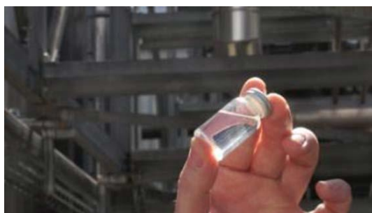
Vial containing isooctane derived from bio-sourced isobutene
