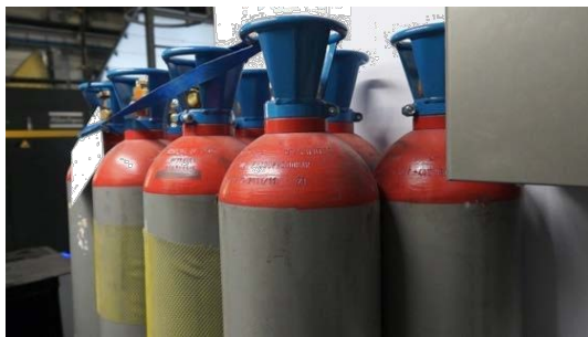
Pressurised containers of liquefied bio-sourced isobutene
