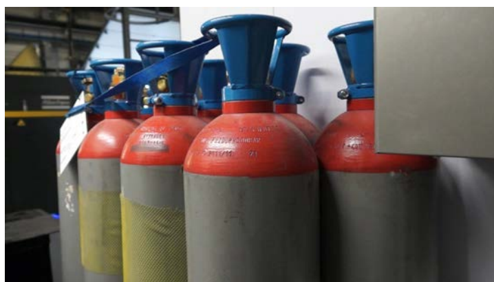
Pressurised containers of liquefied bio-sourced isobutene
